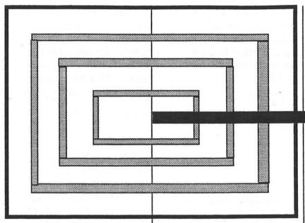
A center loaded system is the best method to hold any size sheet without the possibility of moving. The entire system works by using a vacuum pump, (or a vacuum cleaner) and placing a pipe through the side of the easel and through all of the supports that are glued to the bottom of the easel. Regardless of the size of paper used on the easel, as long as it is centered, the vacuum will hold.
